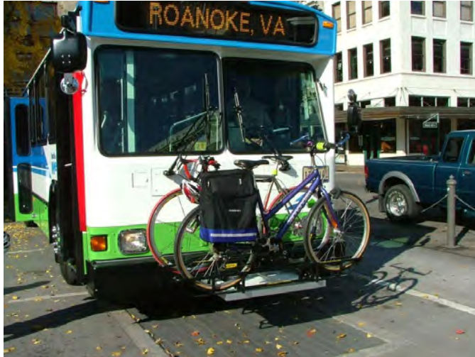
Figure 7.2-1 | The 2006 model Valley Metro buses were the first to feature bicycle racks
